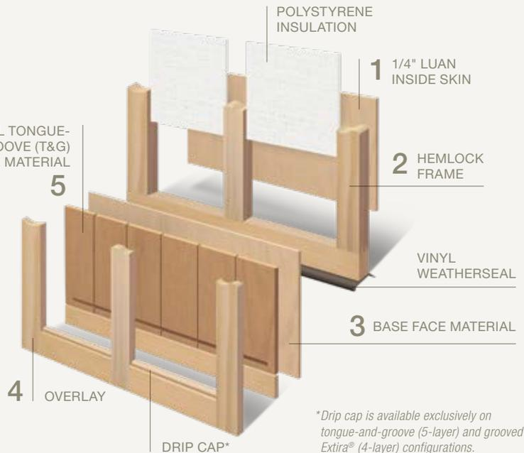
\*Drip cap is available exclusively on tongue-and-groove (5-layer) and grooved Extira® (4-layer) configurations.
